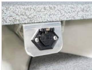
Pre-wired for 12V electric trolling motor.
