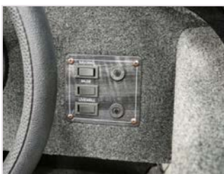
Convenient console switches for your nav lights, bilge pump, and livewell pump.
