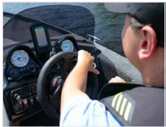
Bluetooth stereo, fish/depth finder, and illuminated gauges and switches.
