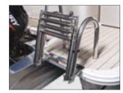
Large telescopic stainless steel boarding ladder makes it easy to climb aboard from a dip in the lake.
