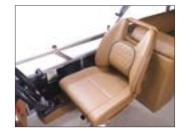
The swivel seat rotates 360° and slides forwards and back.
