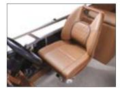
The swivel seat rotates 360° and slides forwards and back.
